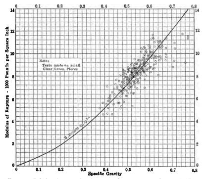
Fig. 22.—Relation between bending strength and dry weight for longleaf pine.
